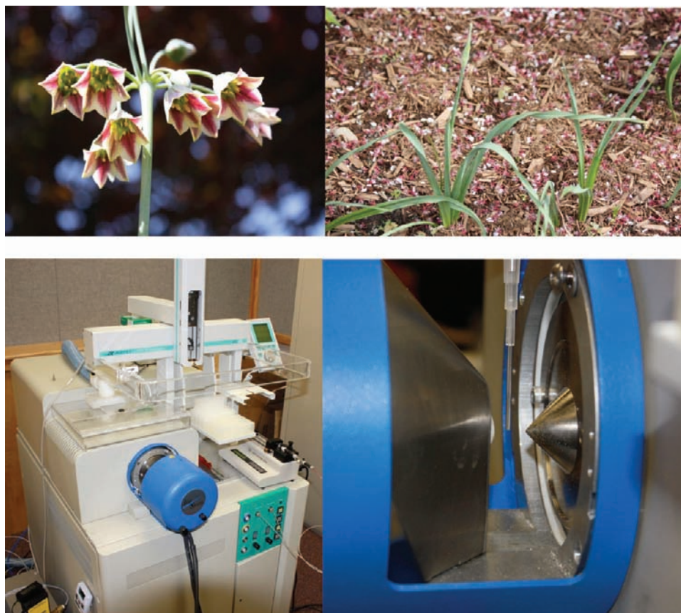
Figure 1. (Top) A. siculum flowers (left) and foliage (right). (Bottom) DART instrument showing autosampler (left) and sample positioned in DART probe (right).
